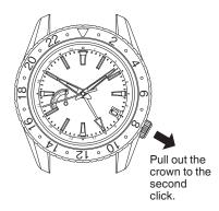
4 Turn the crown counterclockwise (6 o'clock direction) to rotate the 24hour hand and minute hand clockwise and set them to the current time
