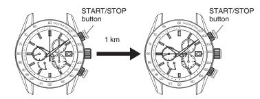
The measured result shows that the average speed of the vehicle is 80 km/h.
