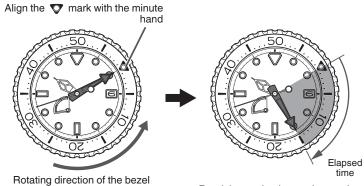
Read the graduation on the rotating bezel to which the minute hand is pointing.
