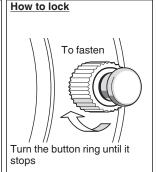
Turn the button ring counterclockwise (6 o'clock direction) to lower the slide cover gradually. Turn the button ring further until you can clearly see the guide line and the button ring can no longer be turned. Now the screwlock type button is unlocked and can be operated.
